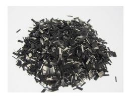
ZOLTEK PX35 Chopped Fiber is commonly compounded with general engineering thermoplastics (e.g., PC, Nylon, etc.) and high-temperature thermoplastic resins (e.g, PEEK, PEI, etc.). The resulting composite offers high strength-to-weight and stiffness-to-weight ratios. Our chopped fibers have a high bulk density value, which allows for cleaner and more consistent flow rates. They also distribute easily during compounding, thereby improving process and product performance.
