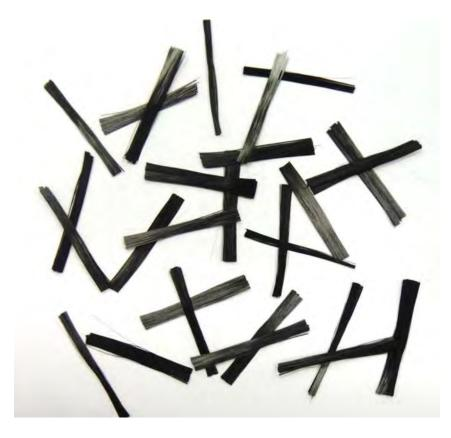
ZOLTEK PX35 KS fiber is ideally suited for Sheet Molding Compound (SMC) applications. Through a proprietary process, the 50K tow bundles are split into 3K sub tows. The resulting KS fiber is designed to be chopped to allow for homogeneous dispersal in SMC for compression molding applications.
