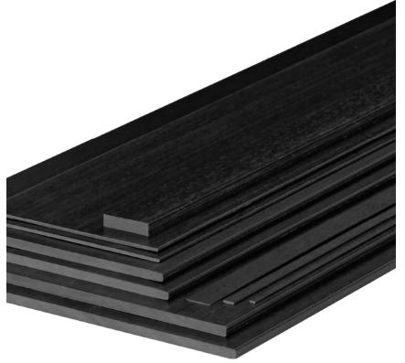
Pultrusion is a cost-effective, continuous process for producing fiber-reinforced composite parts. ZOLTEK PX35 Continuous Tow is fed into our proprietary impregnation and curing process which creates engineered carbon fiber profiles. These profiles enable rapid section buildup when laminating thick parts such as wind blade spar caps. High fiber alignment achieved with pultrusion delivers consistently superior properties in laminates compared to any other composite manufacturing processes.
