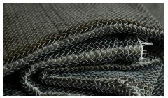
Fabric Weights from 150 - 900 gsm Constructed for Enhanced Infusibility
