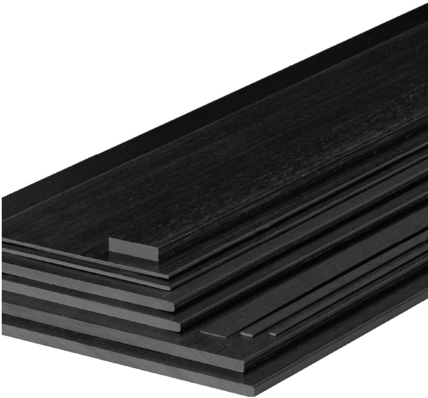
Pultrusion is a cost-effective, continuous process for producing fiber-reinforced composite parts. ZOLTEK PX35 Continuous Towis fed into our proprietary impregnation and curing process which creates engineered carbon fiber profiles. These profiles enable rapid section buildup when laminating thick parts such as wind blade spar caps. High fiber alignment achieved with pultrusion delivers consistently superior properties in laminates compared to any other composite manufacturing processes.
